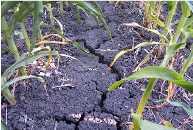
Figure 1. Soil with a high capacity to shrink and swell with drying and wetting.
